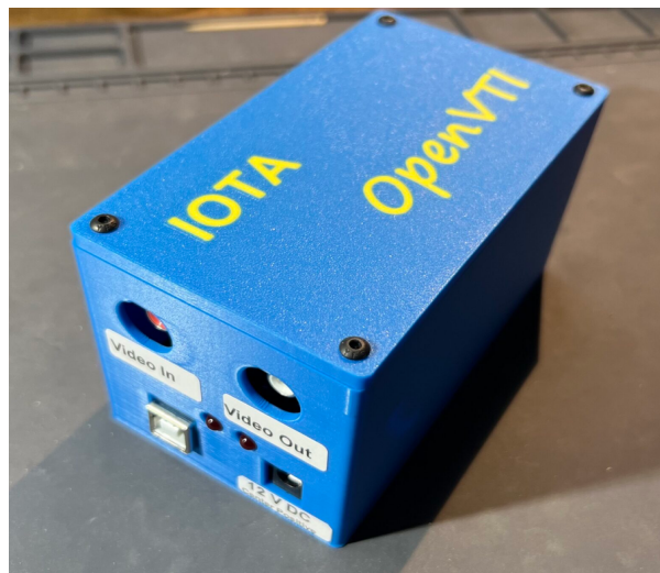
IOTA OpenVTI with connections for power and video. The connector for the GPS antenna is on the backside.
