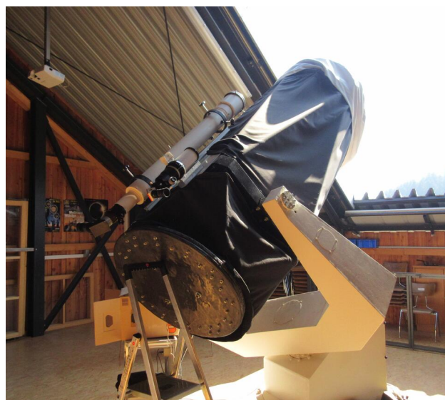
Figure 2. The 60 cm Newtonian on the fork mount inside the spacious Solarstromsternwarte . (Photo: Astronomie im Chiemgau e.V.)
