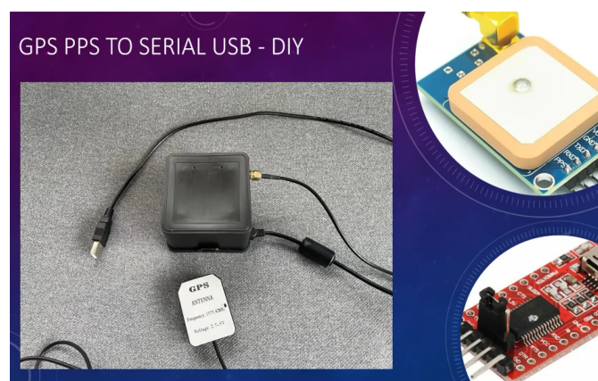
Figure 19. Components of the inexpensive DIY GPS-timing device. (Screenshot from M. Camilleri's presentation)
