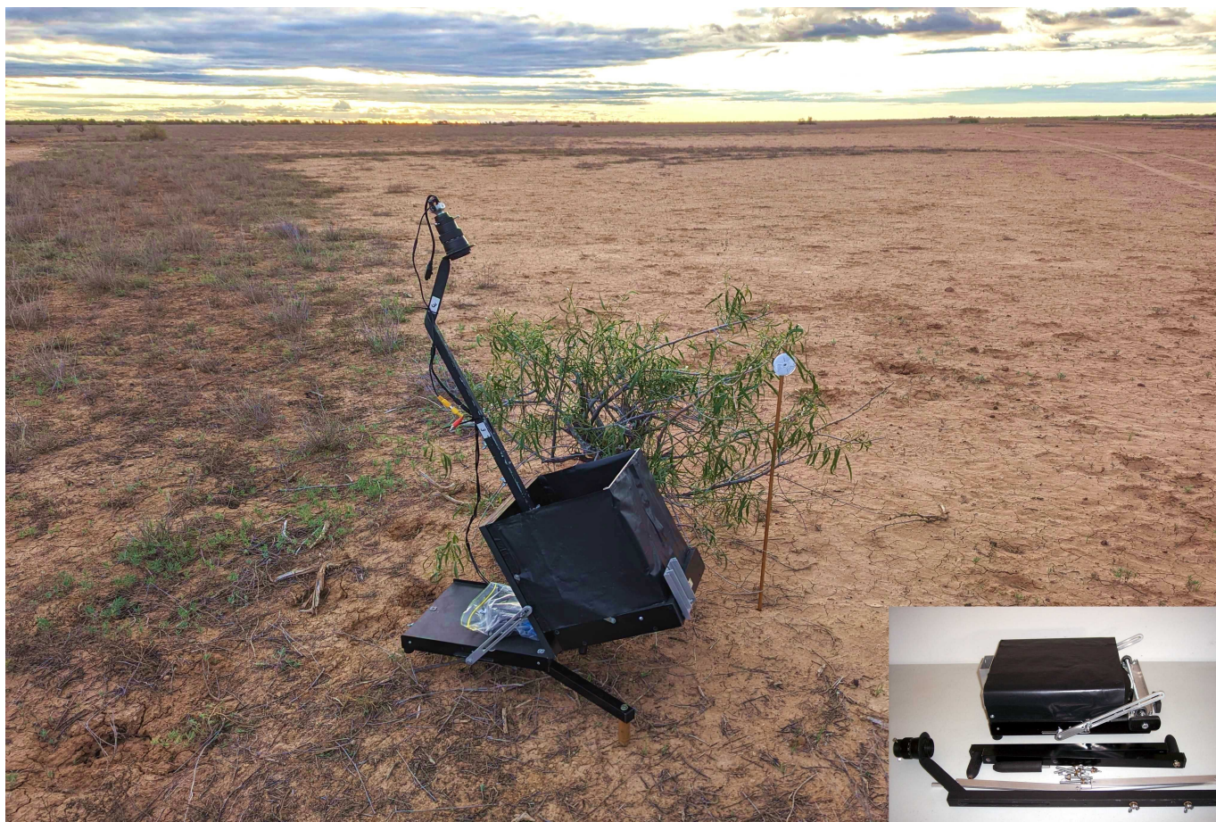
Figure 5. Wombat-250 alt-alt telescope at Station-5 next to a staked reflector for navigation. The inset shows how compact it is in its folded state. Visible at upper right are my own tyre tracks from the previous night's activities, stretching out into the distance.
