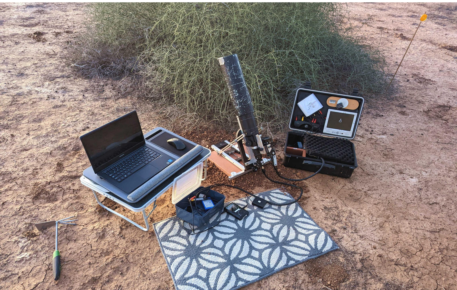
Figure 3. 80 mm refractor mounted on a paver at Station-6 ready for previous-night pointing.
