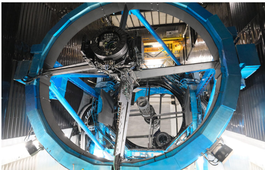
Figure 1. The Hyper Suprime-Cam (HSC) and the primary mirror of the 8.2 m Subaru Telescope . The image of a larger lens of HSC's Wide Field Corrector (WFC) is seen on the primary focus. (Credit: Kazuhito Dobashi/NAOJ)
